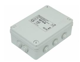
Intelligent Input/Output module for the D-Loop for the control of external optical and acoustic signaling devices with bidirectional isolator according to EN 54-17 and EN 54-18. Including one monitored fault input and one monitored voltage output for signalling devices.
